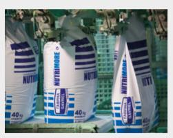
When fed into the filling machine, the tubular FFS film is base-sealed and cut, formed and filled, and then top sealed. The same procedure applies for the flat FFS film, with an extra phase for vertical sealing before base sealing.
